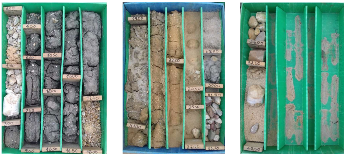
Figure 18- Soil's Profile. Result from the extraction of the borehole close to the Static Load Tests. (Mota-Engil Fundações (2019).
